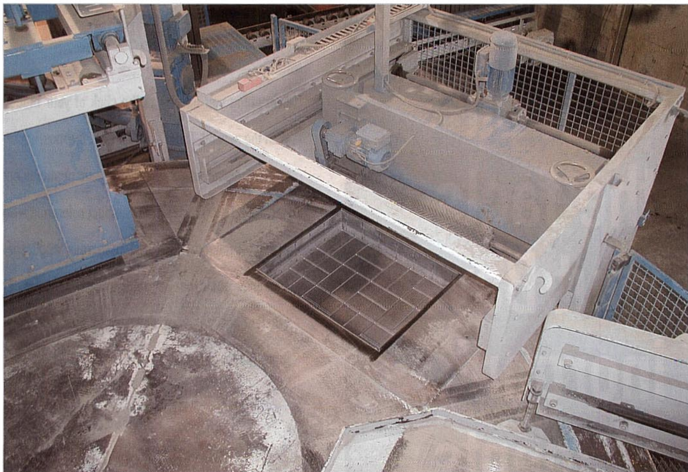
Cobble stone is among the outstanding products from BWS. Here are the matrices of the mould which is adjustable for height.
