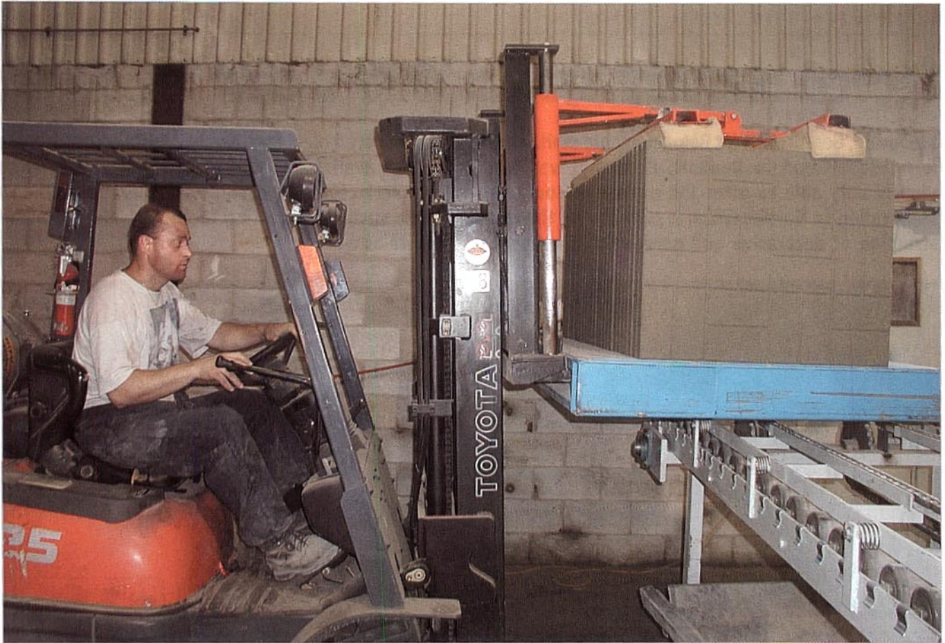
The slabs are driven into the storage area for curing with a forklift while standing on their sides.
