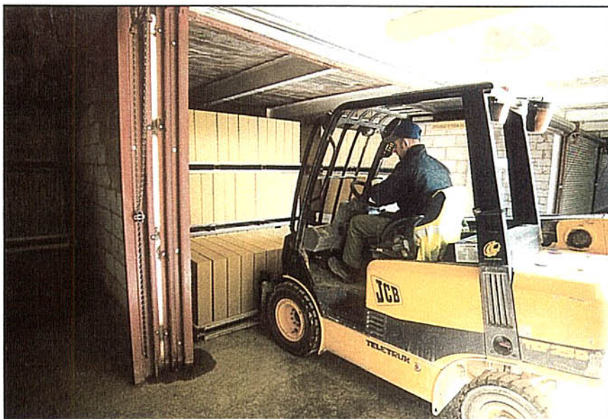
One of the five curing chambers which are adjacent to the press shed.
