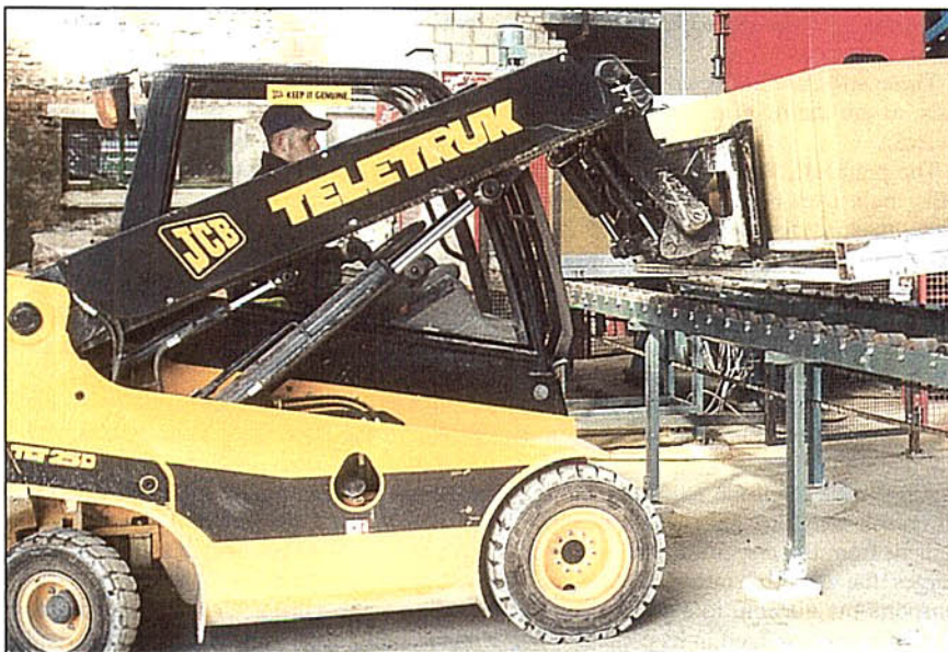
Pallet-loads of slabs are collected by fork-lift for transfer to the curing chambers.
