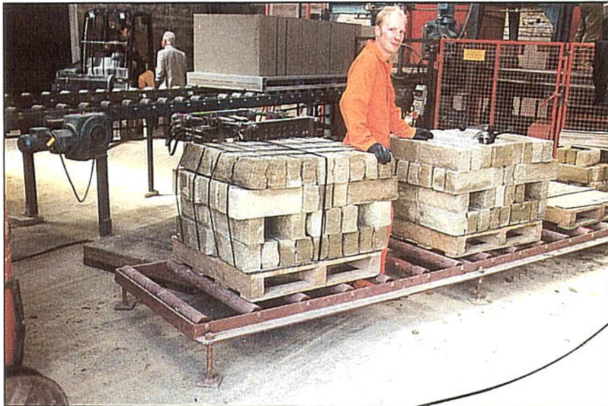
Split stone is packed by hand into cubes, strapped, and then shrink-wrapped.
