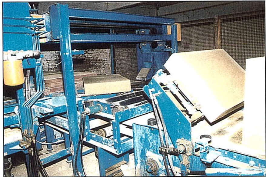
At this turn-table, slabs are edge-stacked for feeding short- or long-face to the splitter.
