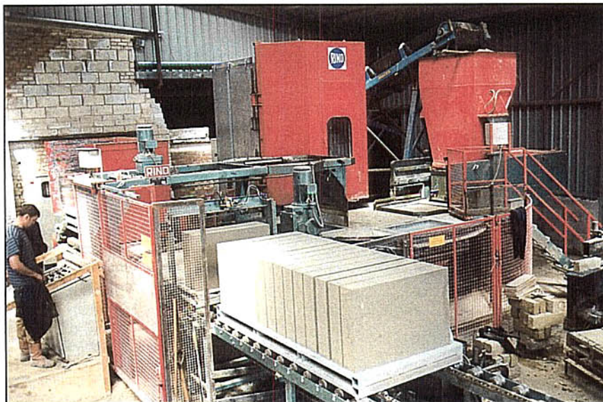
The Rino four-station slab-press at Tudorstone's Ranskill works.
