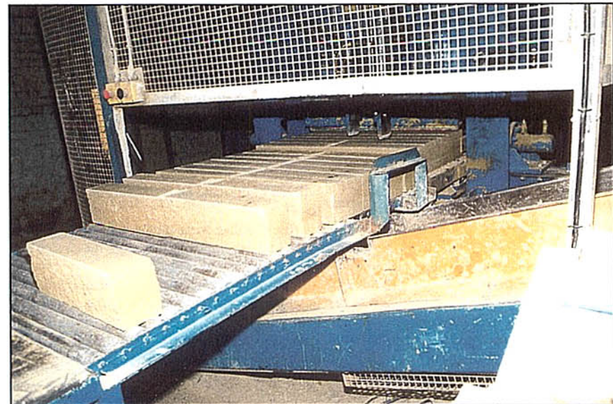
This split stone can be taken into stock or passed through further finishing processes.
